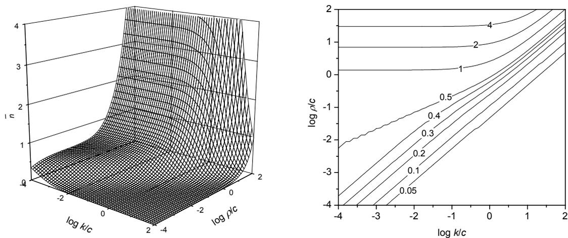
**Figure 6.2:** The 3D surface and contour plot of  $\bar{n}$  vs  $\rho/c$  and  $k/c$  described by the Smith–Ewart equations in steady state where exited radicals have no subsequent kinetic effect. Note the zero-one plateau at  $\bar{n} = 1/2$ .
