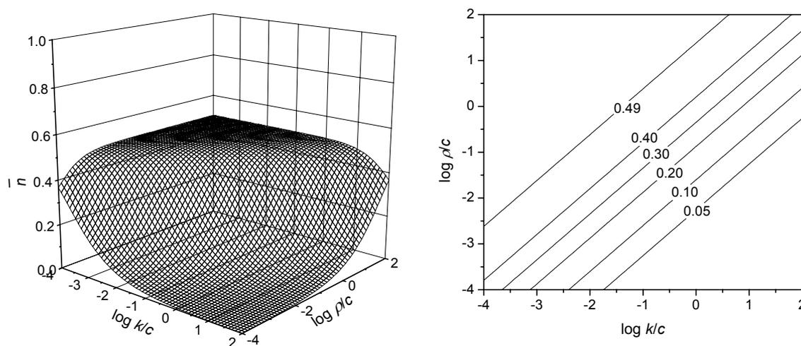
**Figure 6.4:** The 3D surface and contour plot of  $\bar{n}$  vs  $\rho/c$  and  $k/c$  described by the zero-one equations with complete re-entry and minimal re-escape.
