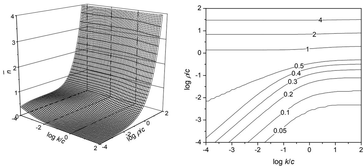
**Figure 6.3:** The 3D surface and contour plot of  $\bar{n}$  vs  $\rho/c$  and  $k/c$  described by the Smith–Ewart equations in steady state with complete re-entry and no subsequent re-escape.
