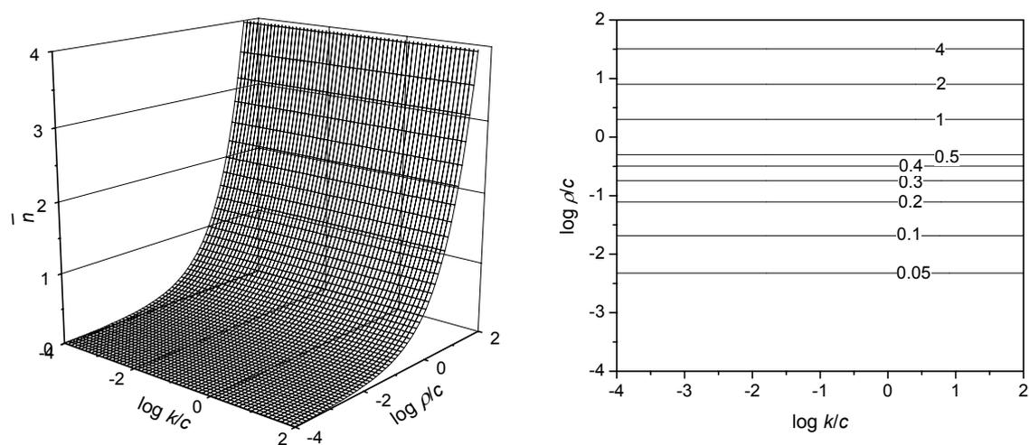
**Figure 6.6:** The 3D surface and contour plot of  $\bar{n}$  vs  $\rho/c$  and  $k/c$  described by the pseudo-bulk equation.
