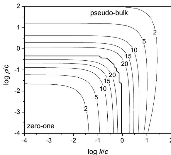
**Figure 6.10:** The best fit to  $\bar{n}$  over the  $(\rho/c, k/c)$ -space with complete re-entry and minimal re-escape, taking  $\bar{n}$  from either zero-one or pseudo-bulk kinetics (selecting on basis of minimum relative error). Contours are of constant percentage error in  $\bar{n}$ . The thick line indicates the boundary between zero-one and pseudo-bulk kinetics being the best fit.
