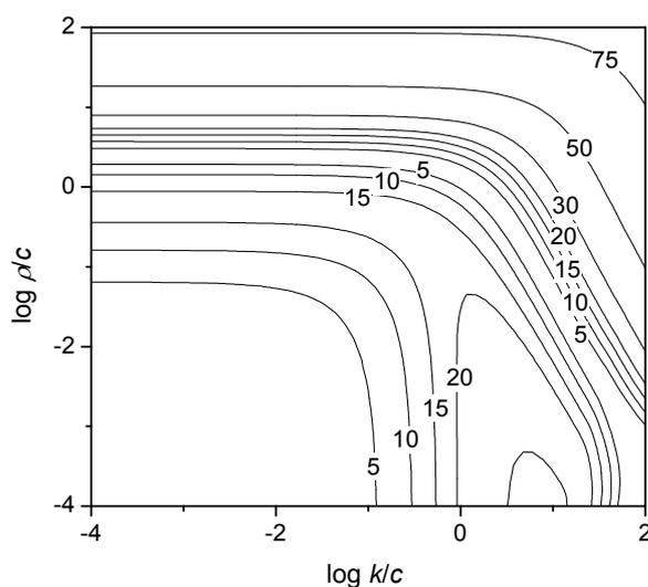
**Figure 6.9:** Percentage error in the calculation of  $\bar{n}$  using zero-one-two kinetics as a function of  $\rho/c$  and  $k/c$  with complete re-entry and minimal re-escape.
