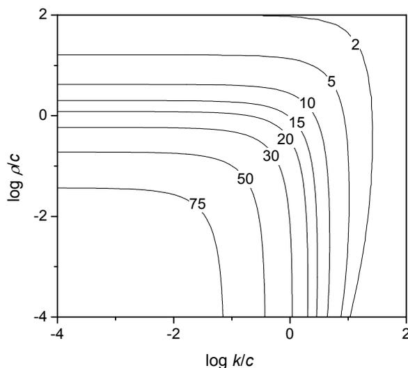
**Figure 6.7:** Percentage error in the calculation of  $\bar{n}$  using pseudo-bulk kinetics as a function of  $\rho/c$  and  $k/c$ .
