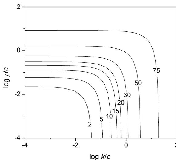
**Figure 6.5:** Percentage error in the calculation of  $\bar{n}$  using zero-one kinetics as a function of  $\rho/c$  and  $k/c$  with complete re-entry and minimal re-escape.
